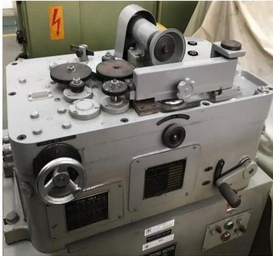
Gambar 3.16 Alat uji keausan *Disk On Block*
