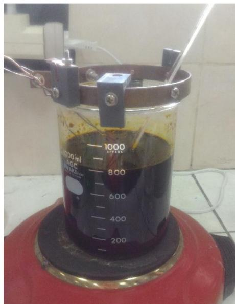
Gambar 3.6 Proses *Chemical Etching*
