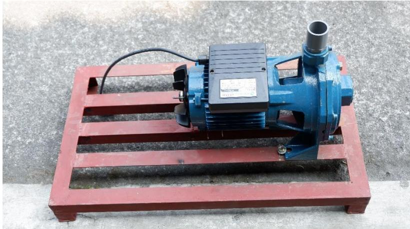
Gambar 3.3. *Monoblock* Pompa Sentrifugal
