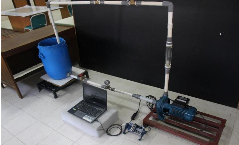
Gambar 3.2 *Test-rig* Kavitasi Pompa Sentrifugal
