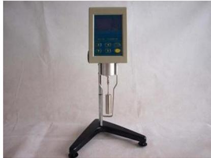
Gambar 2.8 Alat uji viskositas NDJ 8S
