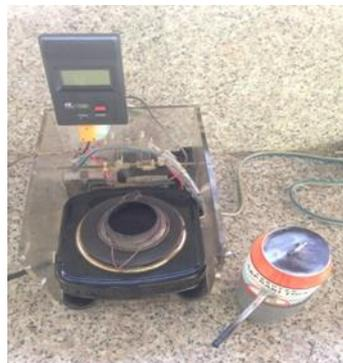
Gambar 2.9 Alat uji *flash point*
