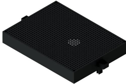
**Gambar 4.10** Desain 3D *Vacuum Chamber*
