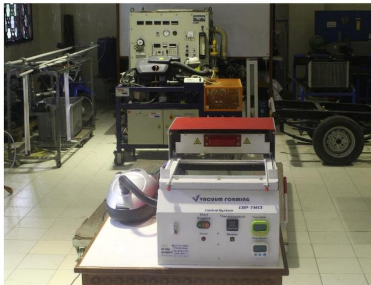
**Gambar 4.39** Mesin *vacuum forming* CRP-TM13
