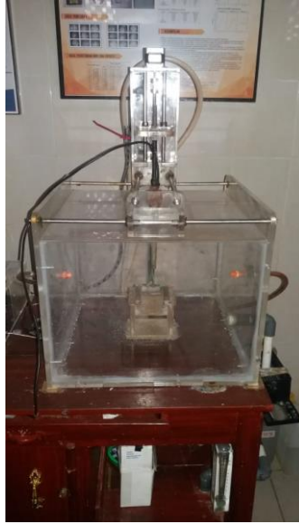
Gambar 3.1 Electrochemical Machining portable single axis.
