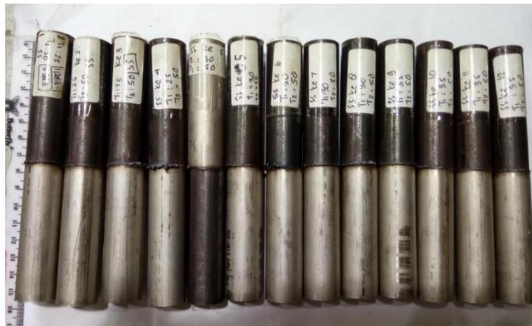
Gambar 4. 1 Hasil Pengelasan Gesek Pipa *Stainless Steel* (Berputar) - Pipa Baja
