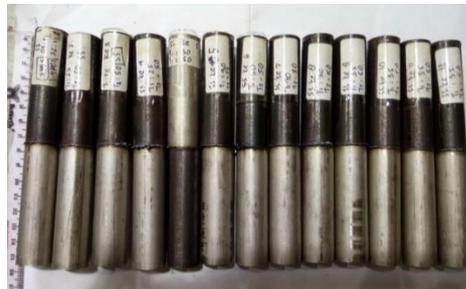
Gambar 4. Hasil Pengelasan Gesek Pipa *Stainless Steel* - Pipa Baja
