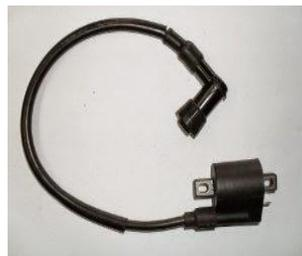
Gambar 3.6 Koil Yamaha YZ 125
