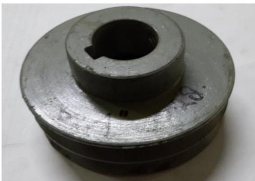
**Gambar 1.4** Pulley diameter 10 cm
