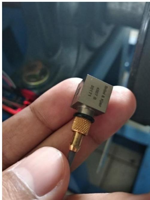
**Gambar 3.10** Akselerometer
