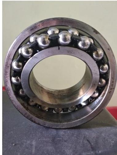
**Gambar 2.8** Bantalan Bola Jenis *Self Aligning Double Row*
