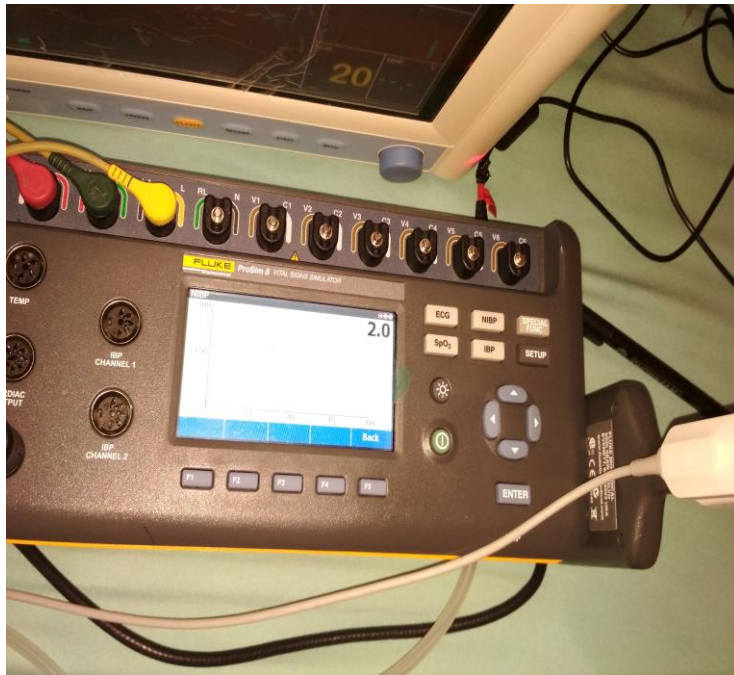
Gambar 3.7 NIBP Simulator Prosim 8
