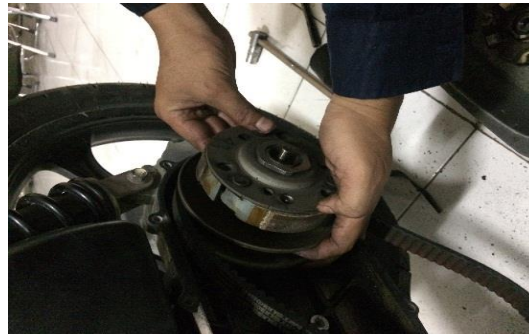
Gambar 3.9 Proses melepas drive belt/V-belt
