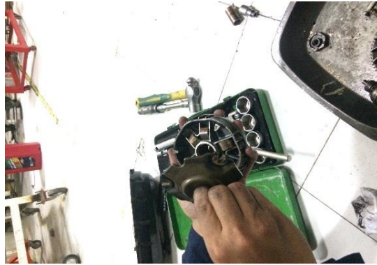
Gambar 3.7 Proses melepas ramp plate
