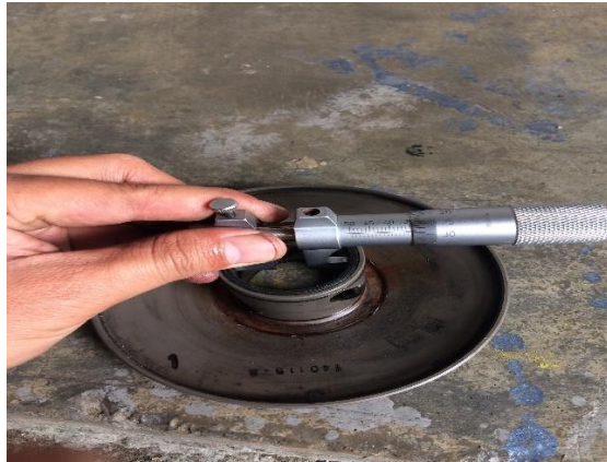
Gambar 3.20 Proses mengukur movable driven face
