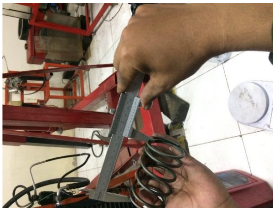
Gambar 3.17 Proses mengukur movable driven face spring
