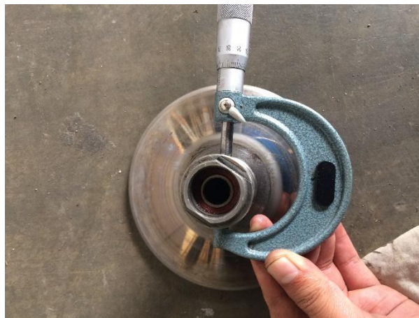
Gambar 3.19 Proses mengukur driven face
