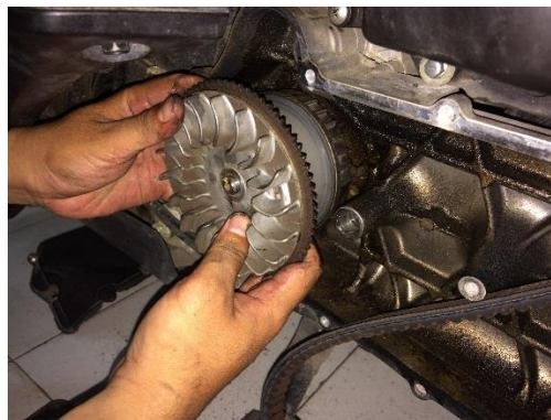
Gambar 3.4 Proses melepas drive pulley face
