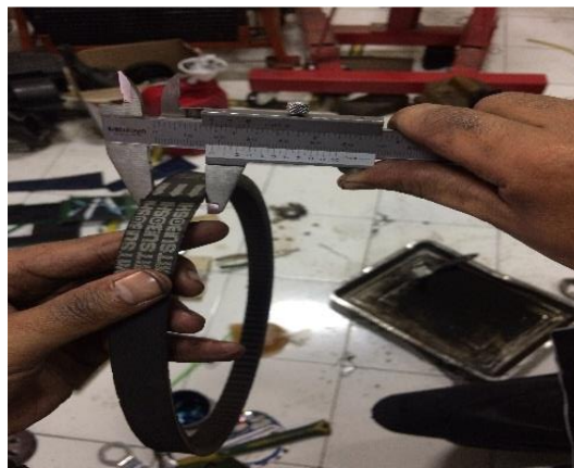
Gambar 3.11 Proses mengukur drive belt
