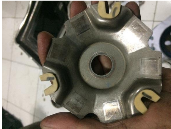
Gambar 3.14 Pengecekan ramp plate
