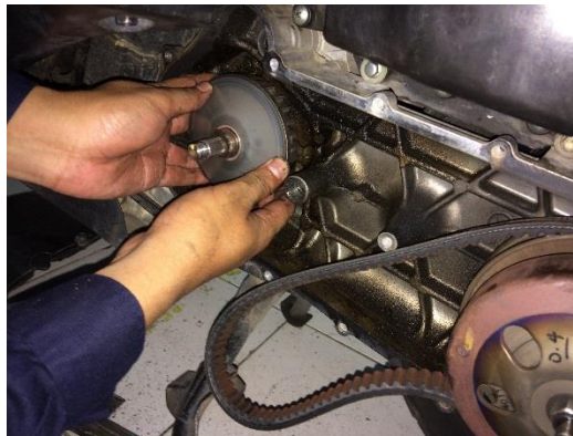
Gambar 3.6 Proses melepas movable drive face
