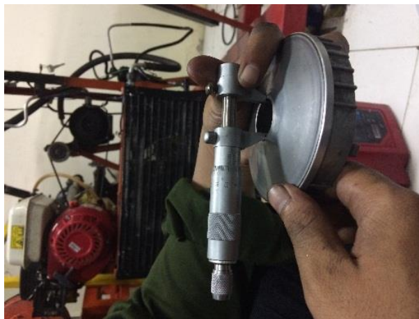
Gambar 3.13 Proses mengukur movable drive face
