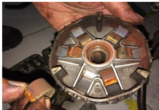
Gambar 3.8 Proses melepas weight roller
