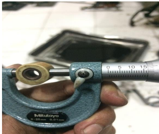
Gambar 3.15 Proses mengukur weight roller
