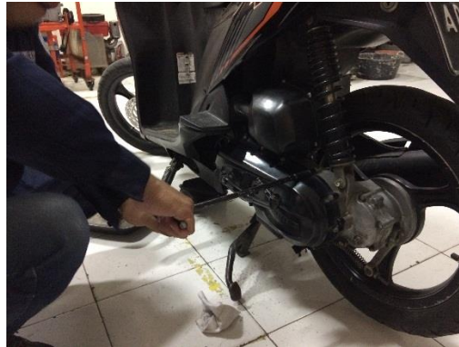
Gambar 3.3 Proses melepas cover CVT
