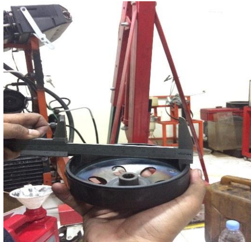
Gambar 3.16 Proses mengukur clutch housing
