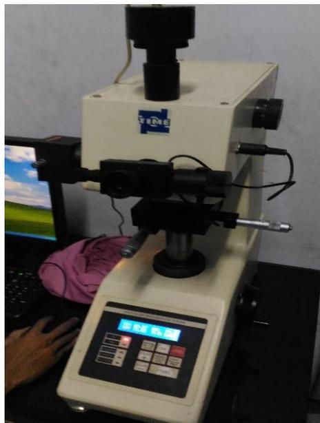
Gambar 4.10 Alat Microhardnest Vicker Tester (Model 402 MVD S/N “V2D531”).
