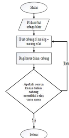
Gambar 3.2 Diagram alur algoritma C4.5
