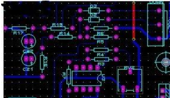
Gambar 3. 18 Lay Out Amplifier
