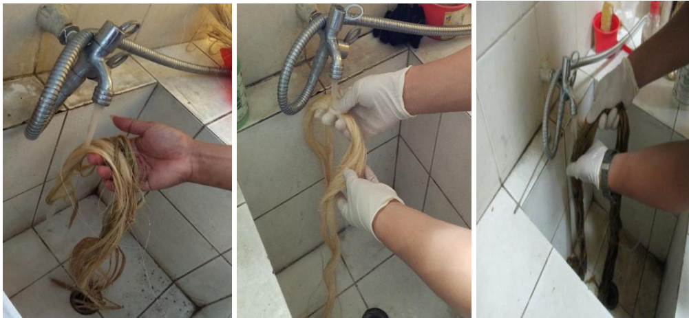
Gambar 3. 25 Proses Pencucian Serat Alam
