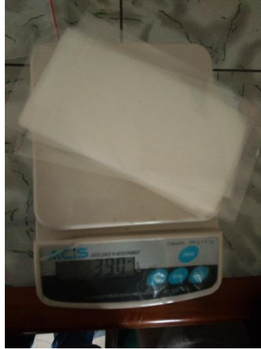
Gambar 3. 38 Proses Penimbangan Matriks
