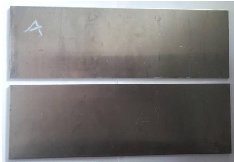
Gambar 3. 1 Bahan Aluminium AA 5083 H116
