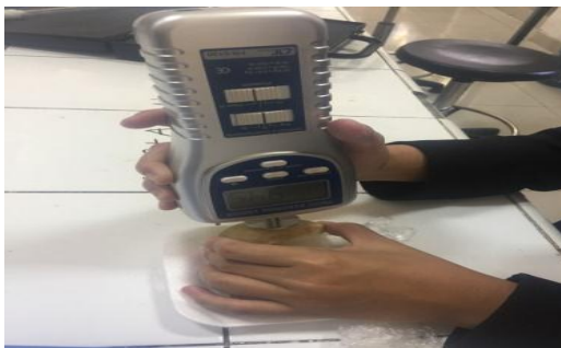
uji kekerasan ( Hand Penetrometer )
