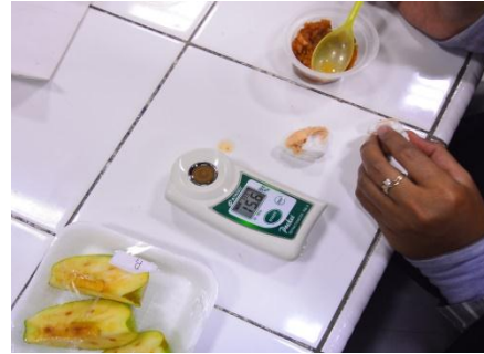
Uji gula total ( hand refraktometer )
