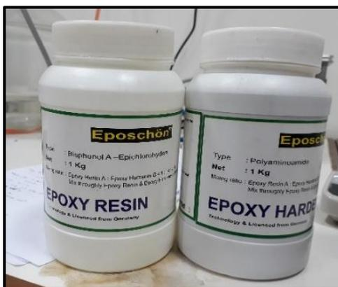
**Gambar 3.3** Epoxy Resin Dan Hardener.
