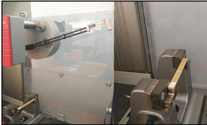
**Gambar 3.11** Alat Uji Impak.
