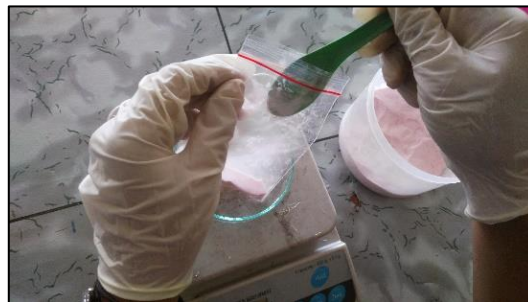
Gambar 3.7 Proses penimbangan PMMA
