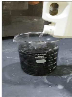
Gambar 3.4 Proses perendaman karbon
