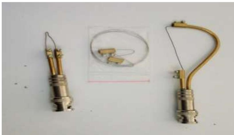
Gambar 2. 3 *Filament Heater.*
