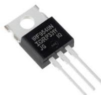
Gambar 2. 3 *Metal Oxide Semiconductor Field Effect Transistor (MOSFET)*
