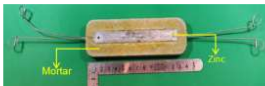
Figure 2: Sacrificial zinc anode F type
