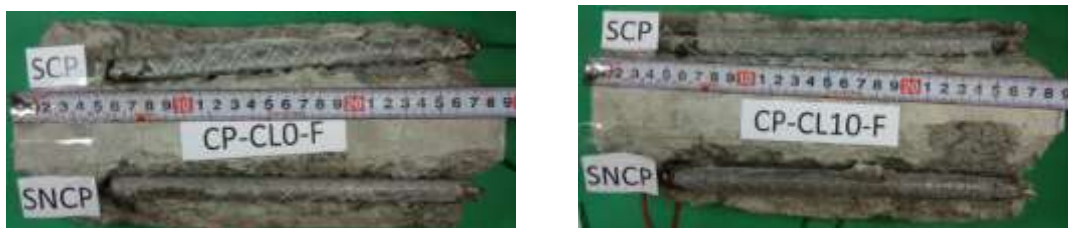
Figure 13: Appearance of rebar corroded area in CP-CL0-F and CP-CL10-F
