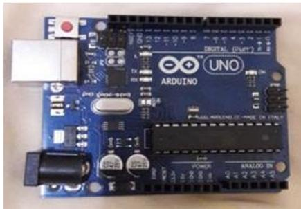
Gambar 2.2 *Board* Arduino Uno
