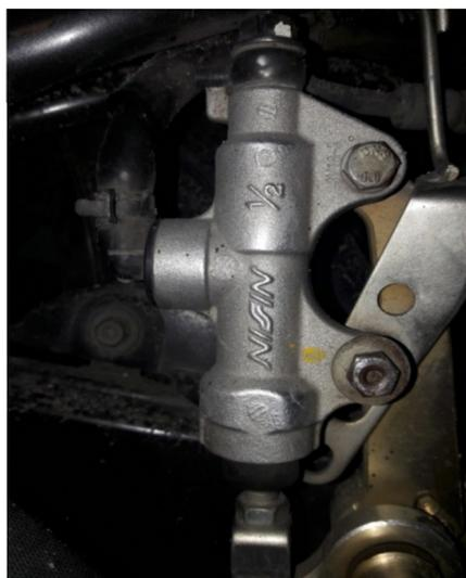
Gambar 2.4 Master silinder sepeda motor
