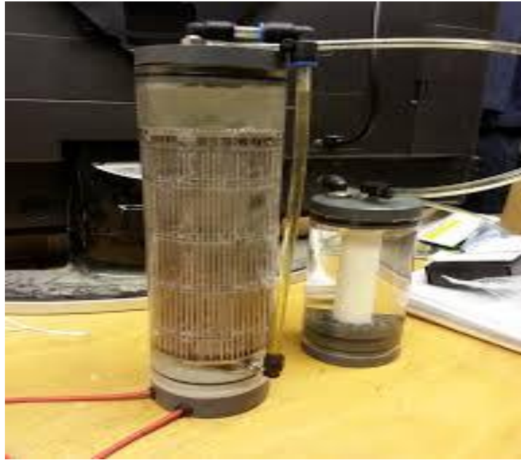
Gambar 2.4. Generator HHO Tipe basa ( wet cell )
