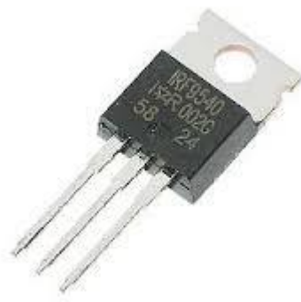
Gambar 2.4 Transistor MOSFET IRF9540[11]
