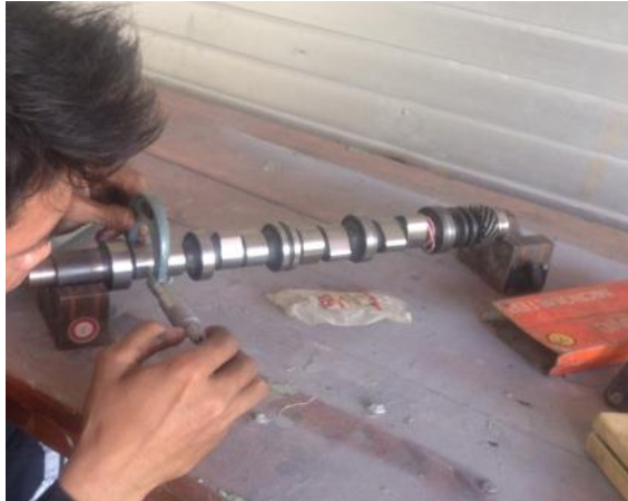
Gambar 4.2.2. Pengukuran Diameter Jurnal camshaft .
