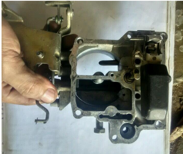
Gambar 4.3 Checking Air Horn / Kepala karburator
