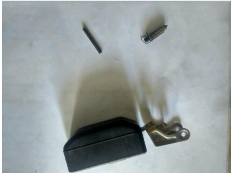
Gambar 4.4 Checking Needle Valve, dan Float
