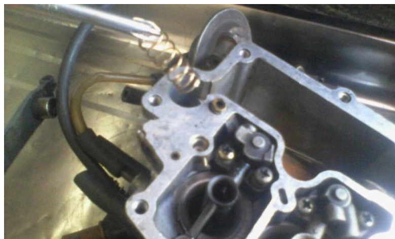
Gambar 3.16 Melepas pump damping spring
