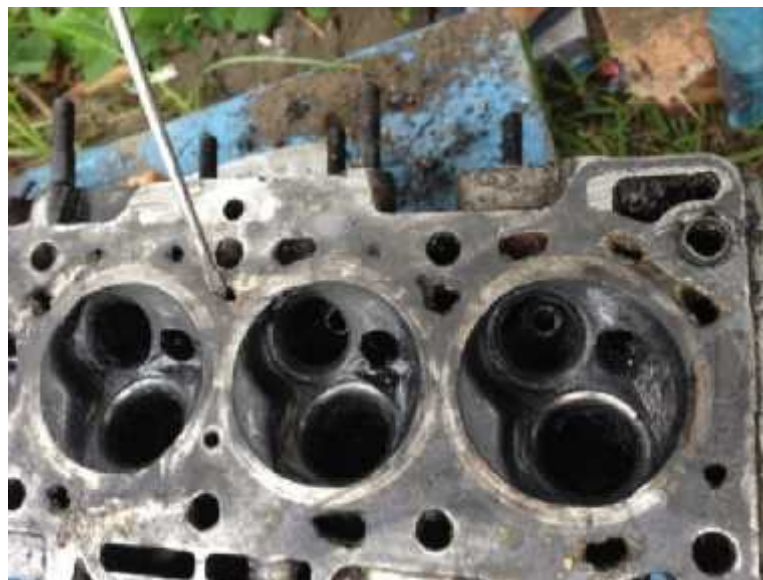
Kedaaan Water Jacket Di Head Silinder
