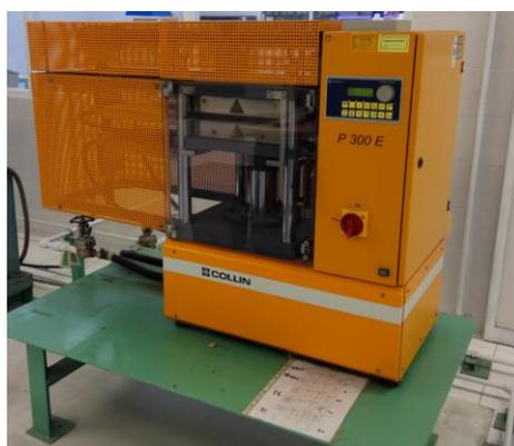
Gambar 1. Hot Press Molding
