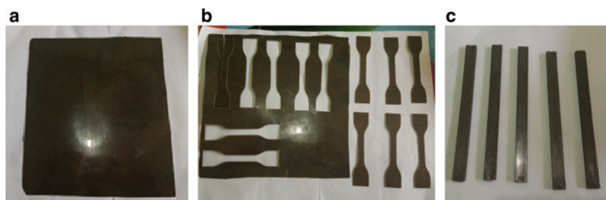
Fig. 1 PVC/FA composite plate (a), tensile test specimen (b), un-notched impact Charpy specimen (c)
