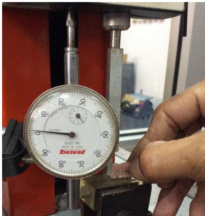
Gambar 13. Uji Tarik Finger Spring
