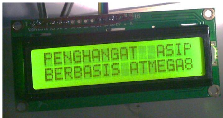
Gambar 2.4. *Liquid Crystal Display (LCD) 16x2*
