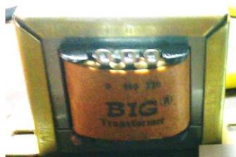
Gambar 2.8. *Transformator 1 Ampere*
