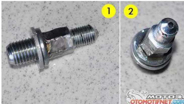
**Gambar 2.11** gambar baut nepel [[www.otomotifnet.com](http://www.otomotifnet.com)]
