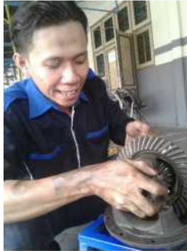
Gambar 4.15 Pemasangan differential case ke differential housing .
