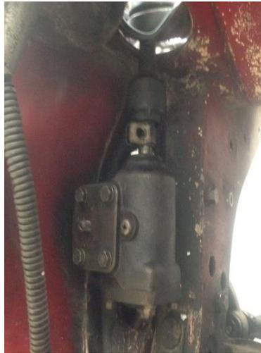
Gambar 4.3 *Recirculating Ball*
