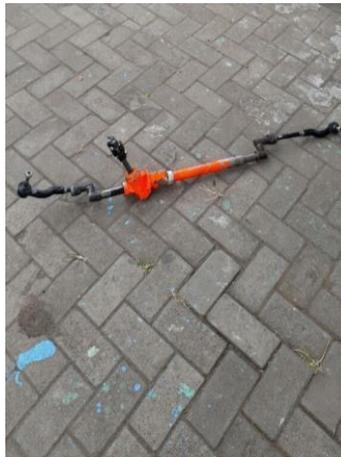
Gambar 4.6 *Steering Linkage Rack And Pinion*
