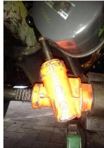
Gambar 4.4 *Rack and Pinion*
