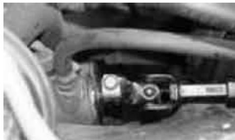
Gambar 2.15 *Steering main shaft*
