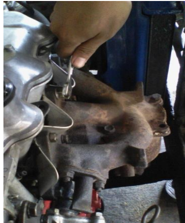
Gambar 3.12 Melepas exhaust manifold
