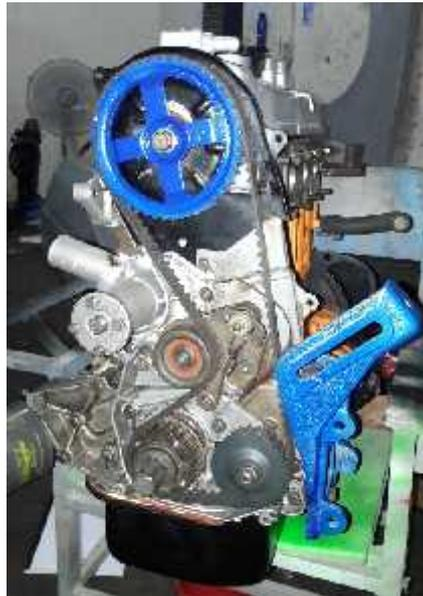
Gambar 4.34. Pemasangan *timing belt*
