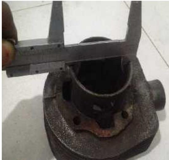
Gambar 4.11 pengukuran diameter silinder
