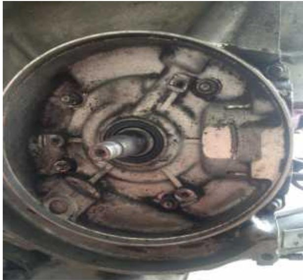
Gambar 3.16 *Seal Crank Shaft*
