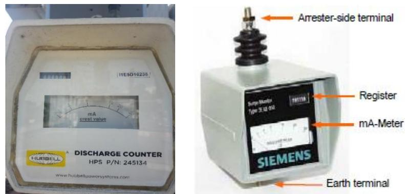
Gambar 2.22 *Discharge counter* dan miliammeter (mA)
