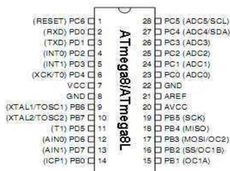
Gambar 2.4 Deskripsi PIN ATmega8
