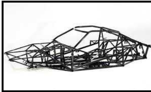
Gambar 2.6 Tipe tubular space frame (alfacell90.blogspot.co.id).
