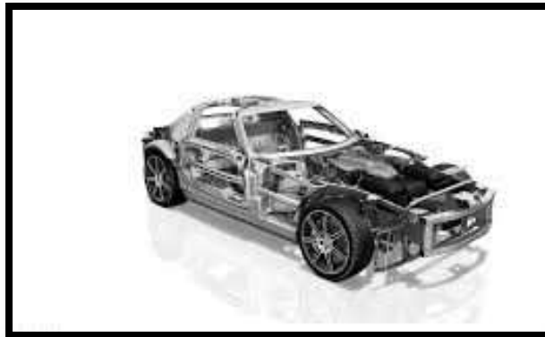
Gambar 2.5 Tipe aluminium space frame (alfacell90.blogspot.co.id).
