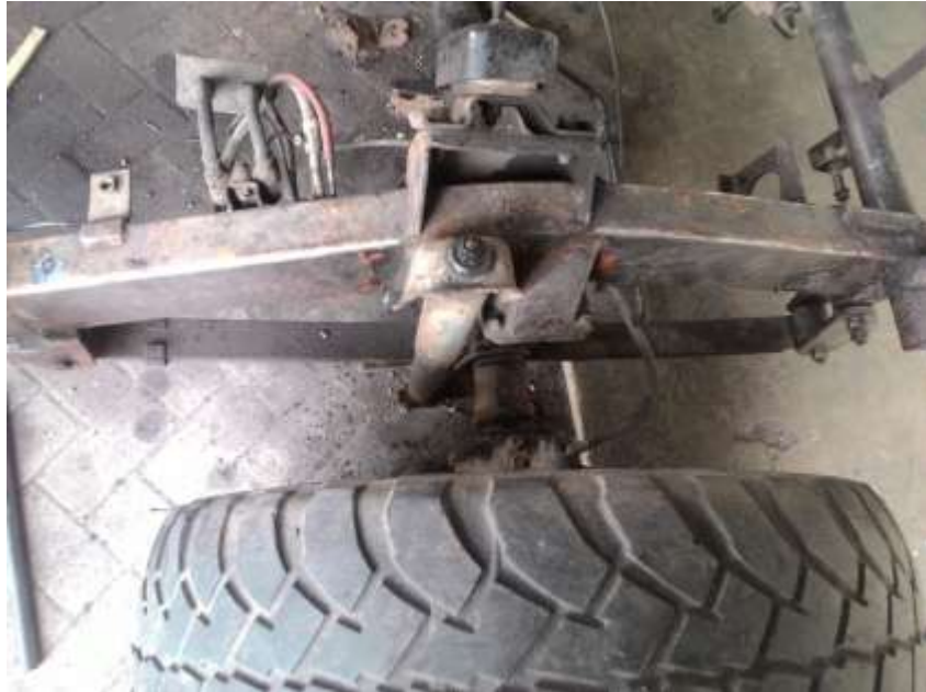
Gambar 4.11 Melepas Shock Absorber
