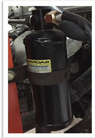
Gambar 4.10 *Receiver/dryer*
