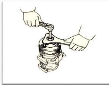
Gambar 3.8 Baut poros (Memelihara/*service* sistem AC,
