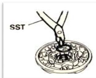
Gambar 3.39 Memasang *snapping* (Memelihara/*service* sistem AC,
