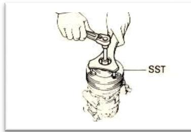
Gambar 3.11 *Pressure plate* (Memelihara/*service* sistem AC,
