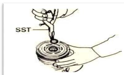
Gambar 3.13 *Snapring* (Memelihara/*service* sistem AC,
