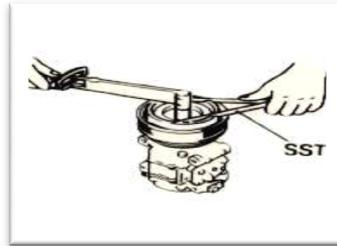
Gambar 3.26 Memasang baut poros (Memelihara/*service* sistem AC,
