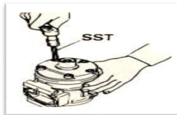
Gambar 3.47 Memasang katup service (Memelihara/*service* sistem AC,
